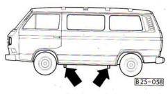
Jack ports - two on each side for front and rear wheel changing.
