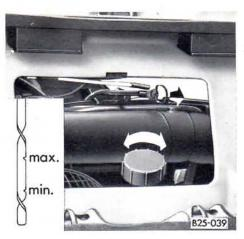
The engine oil dipstick and the oil filler neck are located behind the license plate.
