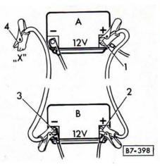
A – DISCHARGED BATTERY B – BOOSTER BATTERY
