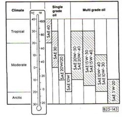
When using single grade SAE 10W or multi grade SAE 5W-20 engine oil avoid high speed long distance driving if outside temperature rises above the indicated limits.
