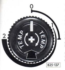
To set the timer, depress the TEMP switch and turn right to the first stop.
