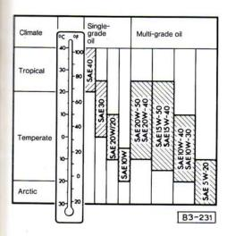
Do not drive with full throttle for long periods when using SAE 10W single-grade oil or SAE 5W-20 multi-grade oil if temperature is above the range shown.
