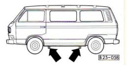
The jack is only designed to lift the vehicle for wheel changing. When working under the vehicle, ensure that it is supported on blocks or trestles.
