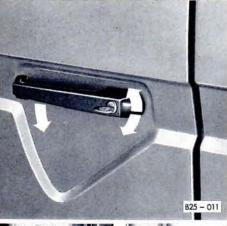
**The sliding door** can only be locked with the key from the outside.
