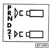
A safety catch is provided for selector lever positions P, R and 1.
