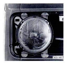
Screw A = Lateral aim Screw B = Vertical aim
