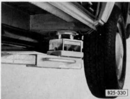
Lifting points for hoist and trolley jack.
