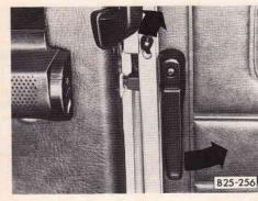
If the sliding door does not close on first try, operate the handle again and pull door back to its fully open position. Do not attempt to use force. You could jam the door and damage the sliding mechanism.
