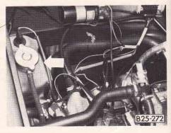
Expansion tank Gasoline engine
