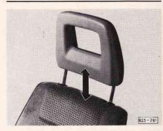
■ For height adjustment grasp head restraint with both hands and pull up or push down.
