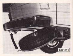
■ When re-installing the spare wheel, slide spare wheel onto metal plate.
