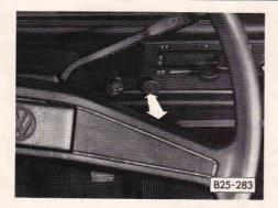
■ If engine does not start, wait for about 30 seconds, switch glow plugs on again and start as described.
