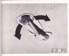
**To open** pull crank handle out of recess and turn counter-clockwise.
