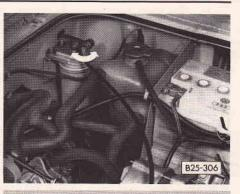
Open vent screw at top of fuel filter.
