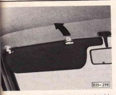
You can lift the visor on the driver's side out of the center mounting and move it toward the door window to protect against side glare.
