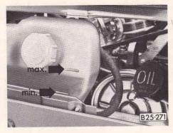
Refill tank Gasoline engine
