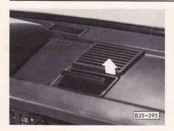
To **remove** ashtray from **dashboard**, grip the strip on opened lid and lift at one side to take out.
