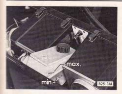
The brake fluid reservoir is located under the instrument cluster in the dashboard canel.
