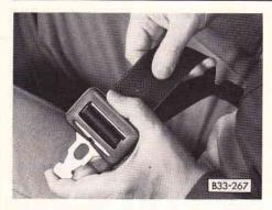
■ To fasten lap belt, grasp belt tongue on outboard side of seat, pull across pelvis and insert in inboard buckle.
