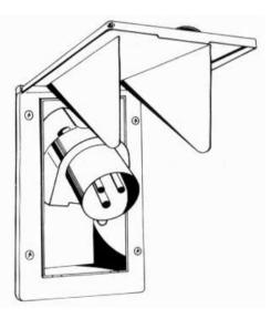
The external socket 220v – 16 Amps to CEE 17 (European Standard) is located on the external left hand side of the vehicle.
