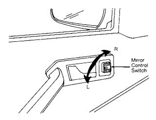
Fig. 1: Controlling Mirror Switch
