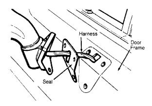
Fig. 11: Installing Mirror Assembly (Vanagon) Courtesy of Volkswagen United States, Inc.
