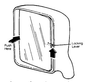
Fig. 6: Removing Mirror Glass (Vanagon)
