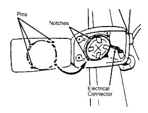
Fig. 3: Installing Mirror Glass (Corrado & Passat) Courtesy of Volkswagen United States, Inc.
