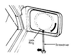
Fig. 4: Removing Mirror Glass (Golf GL, GTI, Jetta & Jetta GLi) Courtesy of Volkswagen United States, Inc.
