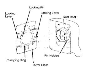
Fig. 7: Installing Mirror Glass (Vanagon) Courtesy of Volkswagen United States, Inc.
